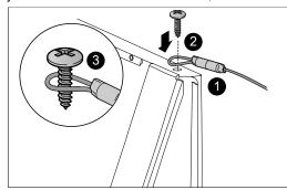
4. retighten the screw complete with the cable on the roof of the appliance;
