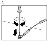
The cable must then be fixed to the wall with a plug, to permanently secure the appliance;
