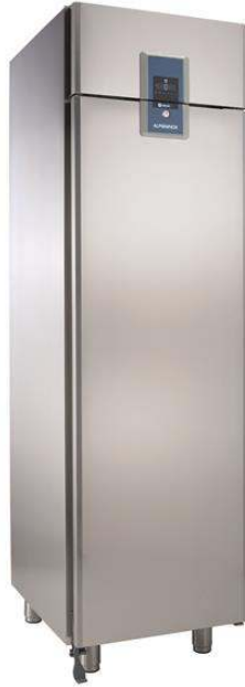
1-door prostore refrigerator 470L, 0+10°C, (R290), AISI 304
