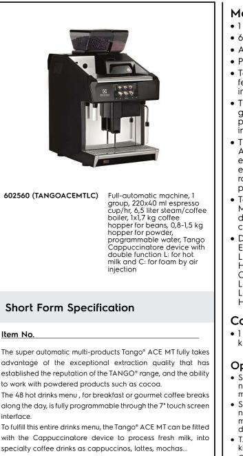
**Delivery Capacity:** Espresso 40ml: 220 cups/h Lungo 100ml: 150 cups/h Hot chocolate 250ml: 110 cups/h Cappuccino 100ml: 170 cups/h Latte 100ml: 150 cups/h Latte macchiato 300ml: 80 cups/h Hot Water: 30 L/h
