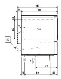
Drain Electrical inlet (power)
