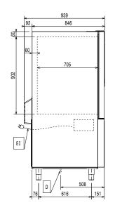
Drain Electrical inlet (power)
