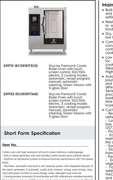
Programs (a maximum of 1000 recipes can be stored and organized in 16 different categories); Manual (steam, combi and convection cycles); Specialistic Cycles (regeneration, Low Temperature Cooking, proving, EcoDelta, Sous-Vide, Static-Combi, Pasteurization of pasta, dehydration, Food Safe Control and Advanced Food Safe Control)
