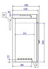
= Drain D ΕI = Electrical inlet (power)
