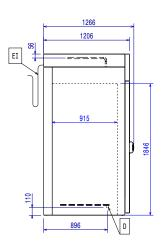
ΕI = Electrical inlet (power) = Refrigerant Outlet RO
