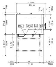
C-WI-Cold Water inlet 1 ΕI Electrical inlet (power)
