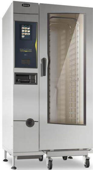
218774 (ZCOG201T2U0) Magistar Combi TS combi boiler oven with touch screen control, 20x1/1GN, gas, 3 cooking modes (automatic, recipe program, manual), automatic cleaning (Australia)
