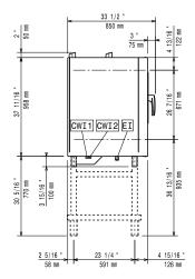
C-WI-Cold Water inlet 1 **EI** = Electrical inlet (power)
