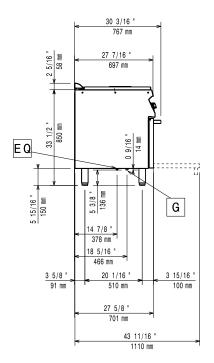
EQ = Equipotential screwG = Gas connection
