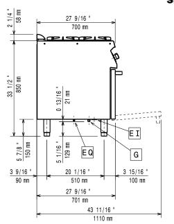
EI = Electrical inlet (power)G = Gas connection
