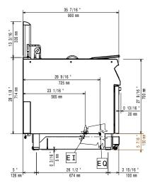
EI = Electrical inlet (power) **EQ** = Equipotential screw
