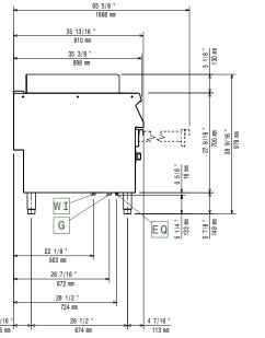
EQ = Equipotential screwG = Gas connection
