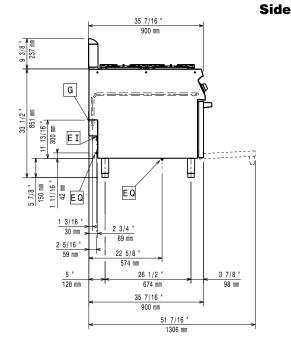
EI = Electrical inlet (power) Gas connection
