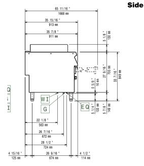
EQ = Equipotential screwG = Gas connection
