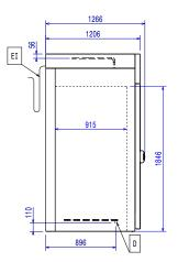
= Drain D Electrical inlet (power)
