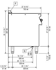
EQ = Equipotential screwG = Gas connection
