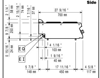
EI = Electrical inlet (power) Equipotential screw =
