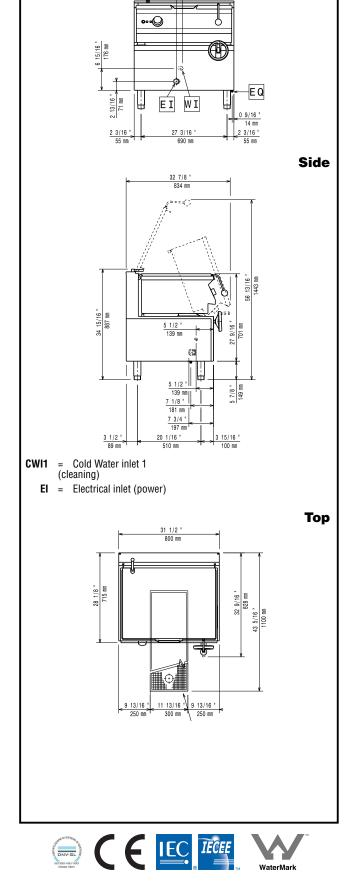
Modular Cooking Range Line EVO700 Electric Tilting Bratt Pan 60lt with Duomat bottom
