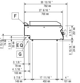
EQ = Equipotential screwG = Gas connection
