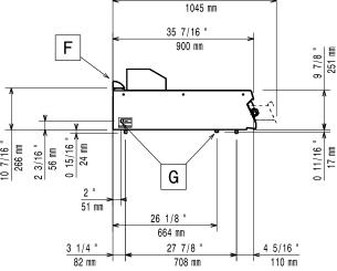
EQ = Equipotential screwG = Gas connection
