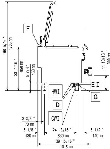
**CWI1** = Raccordement eau froide    **HWI** = Raccordement eau chaude
