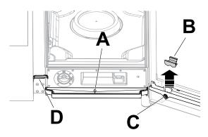
3. Use regularly a pipe cleaner with nylon bristles (supplied with the appliance, according to the model) to clean the small gutter ("D").
