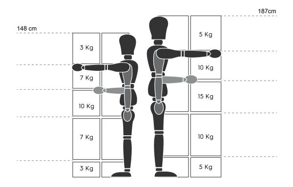
Maximum suggested weighs - "Manual Handling Operations Regulations" - Health and Safety Executive (HSE, UK, 2016) Below a few examples of common installations and the maximum suggested weights per trays
