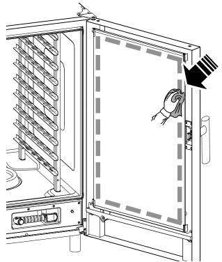
With the door open, press the two top and bottom retaining clips as shown in the figure to reach the intermediate space between the inner and external glass; Clean the outer side of the internal glass door using a glass product;
