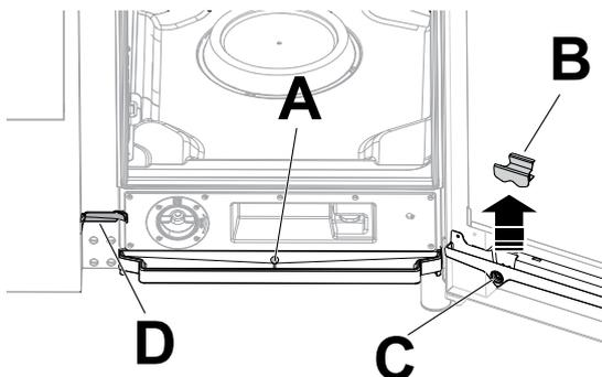
3. Use regularly a pipe cleaner with nylon bristles (supplied with the appliance, according to the model) to clean the small gutter ("D").
