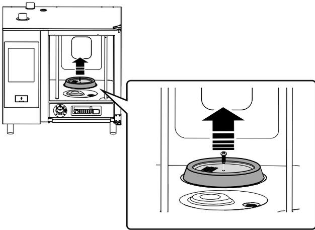
2. Remove the filter from its housing;
