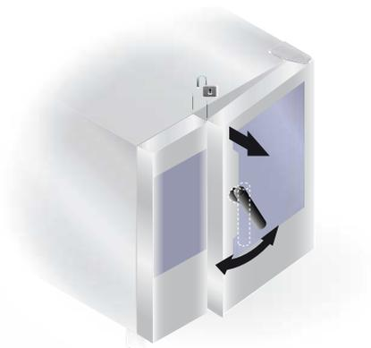
1. Turn the door handle clockwise or counterclockwise all the way to fully open the oven door. The cooking cycle is stopped, if in progress.
