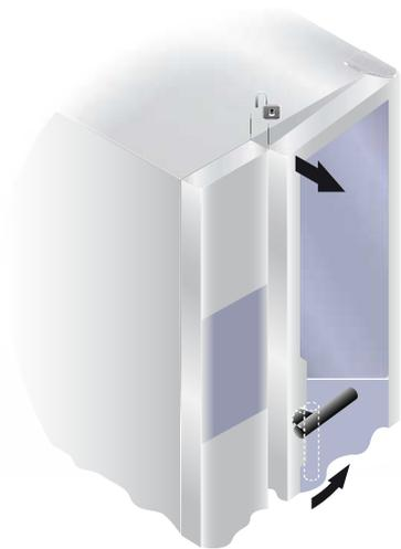
1. Rotate the handle by 90°C counterclockwise to open the door completely. The cooking programme is stopped, if in progress.
