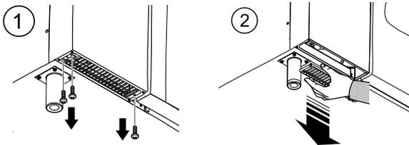
2. Remove the filter and degrease it by washing it with dish detergent;
