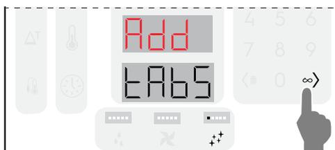
Press button to confirm the solid chemical loading.
