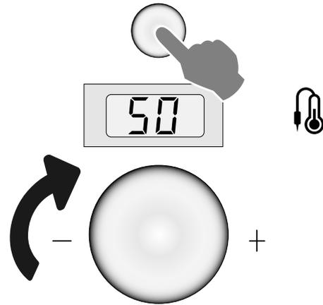
The cooking cycle now starts and continues until the actual core temperature of the product shown on display reaches the programmed core temperature.
