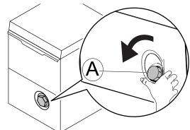
• Pour approximately 0.5 Kg of coarse salt [NaCI] (the amount necessary to fill the salt container up to the rim) into container "**A**".
