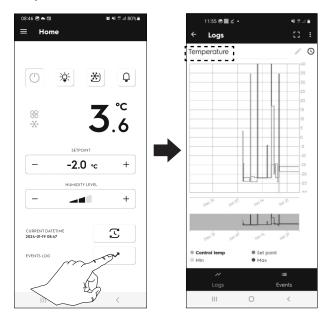
The graphic shows data about temperature, min or max and set point.
