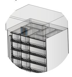
To allow good air circulation and correct uniformity in the compartment, make sure the trays (or other) do not to obstruct the air inlet and delivery duct.
