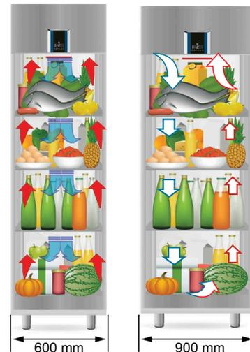
In case of excessive product loading, the temperature remains uniform thanks to the removable rear supports which act as an air conveyor.
