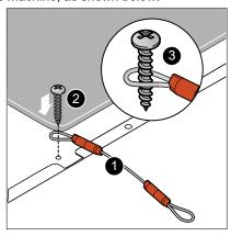
4. retighten the screw complete with the cable on the roof of the appliance:
