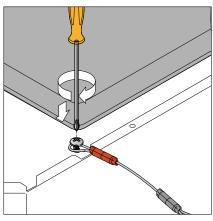
5. the cable, must then be fixed to the wall using a plug, to permanently secure the appliance.
