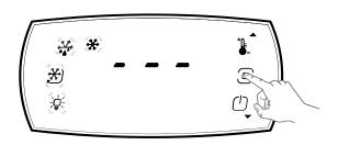
Press the temperature button. The display shows the SET POINT.
