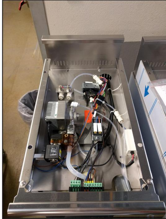
3- Disconnect the main connector on the back. Unscrew (not fully) the two screws; then simply slide the unit forwards to extract the module.
